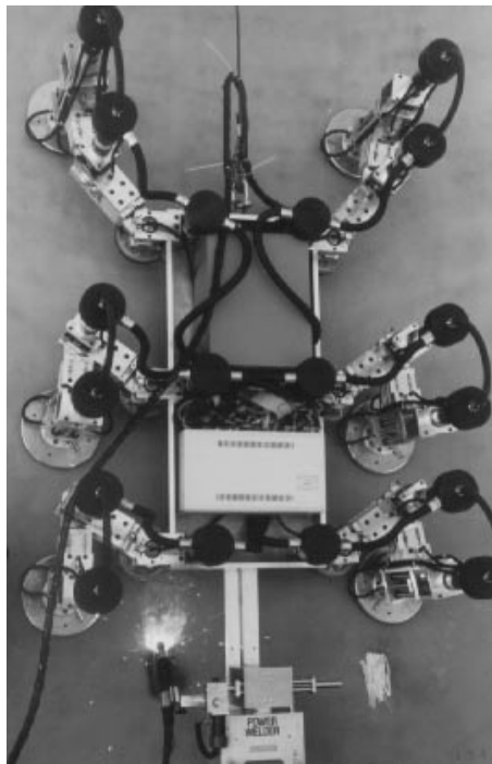
Figure 12. REST 1 climbing robot welding ship hull.
