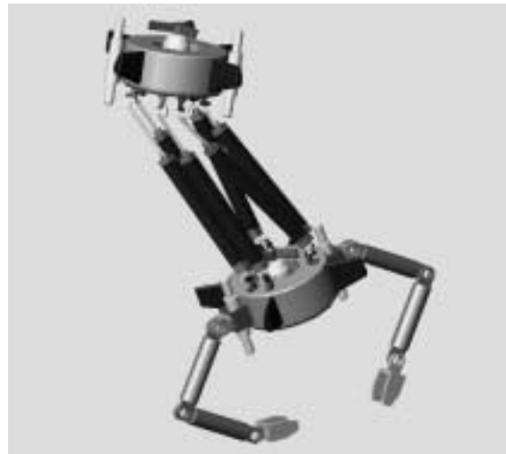
b) UPR for underwater manipulations works.
