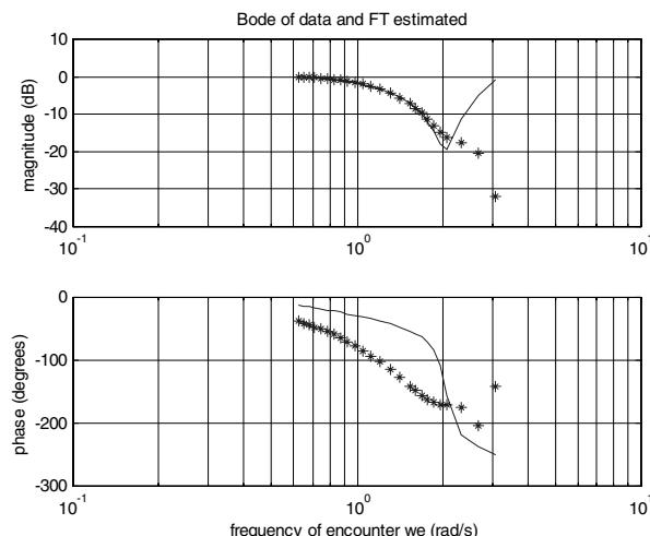
Figure 3.Bode plot of  $G_{1H}(s)$  and experimental data
